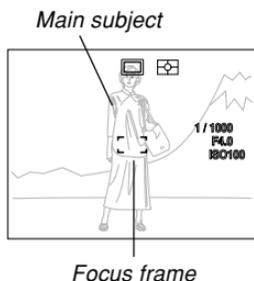
2. Keeping the shutter button pressed half way down, re-compose the image as you like.
